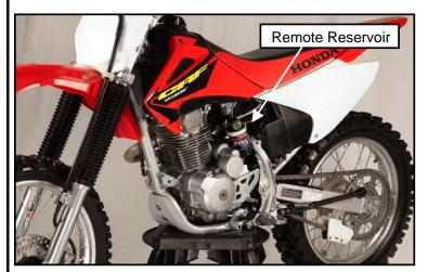
The CRF 150/230F Podium X you purchased from Fox Racing Shox is different from Honda's stock unit, as it is completely adjustable and has a remote oil reservoir that is mounted to the frame. Installation is not as simple as the stock shock, so please carefully follow the instructions below to ensure safe operation.
